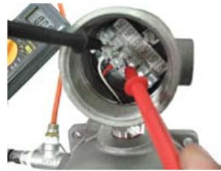
7. If the range needs to be reseted, please open an upper cover at first and relax the revolvable cam with the hexangular key wrench. Turn the pointer to the requested alarm set point with hand and hold the hand at the position.Let the revolvable cam touch the micro switch to cause NO, COM short-circuited. When the multimeter displays zero,lock the cam tightly in place.
