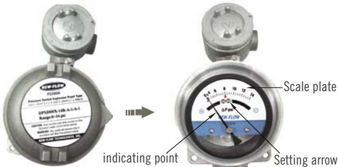
2. Leakage Test : Given a pressure in high side and low side at same tim for check leakage to connection (according to working pressure rate) (Fig 2)
