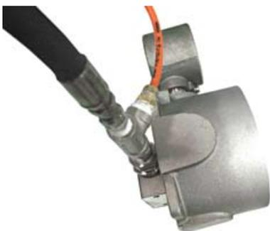
5. Scale range check : Given a pressure limited to maximum scale range: then increase pressure into low side confirm  $\Delta P$  range is correct. (Fig 5)
